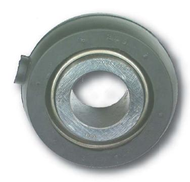
NTN-BCA CDS assemblies are designed specifically for tillage applications with high shock loads. The CDS units are comprised of an integral bearing and a rubber grommet housing that absorbs impact loads.
